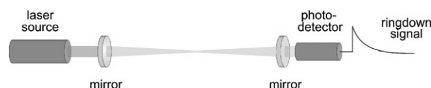
Fig. 1 Schematic of a cavity ringdown spectrometer (see text for explanation). A stable cavity is obtained by employing plano-concave mirrors with a radius of curvature chosen to re-focus the light on each reflection.
